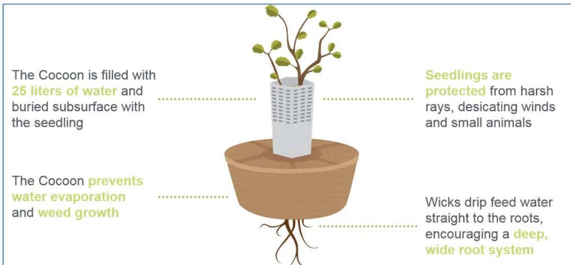
Figure 1. Scheme of the Cocoon device
