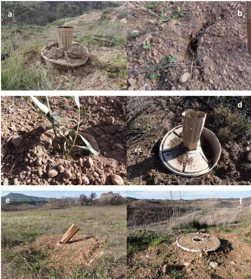
*Symptoms of deficient installation or devise limitations or failures: Cocoon outstanding from soil surface (a); incorrect fulfill of holes (space between Cocoon and soil walls) (b); excessive fulfilling of seedling holes (c); lip collapse (d); protector fall (e); protector lost (f).*
